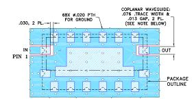
NOTE: 1. COPLANAR WAVEGUIDE PARAMETERS ARE SHOWN FOR ROGERS RO4350B WITH DIELECTRIC THICKNESS .060" ± .004"; COPPER: 1/2 OZ. EACH SIDE. FOR OTHER MATERIALS TRACE WIDTH MAY NEED TO BE MODIFIED. 2. BOTTOM SIDE OF THE PCB IS CONTINUOUS GROUND PLANE. DENOTES PCB COPPER LAYOUT WITH SMOBC (SOLDER MASK OVER BARE COPPER) DENOTES COPPER LAND PATTERN FREE OF SOLDER MASK E
