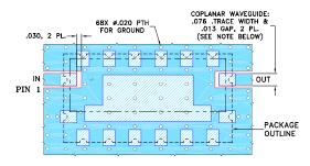
NOTE: 1. COPLANAR WAVEGUIDE PARAMETERS ARE SHOWN FOR ROGERS RO4350B WITH DIELECTRIC THICKNESS .060" ± .004"; COPPER: 1/2 OZ. EACH SIDE.
