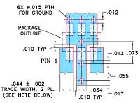
NOTE: 1. TRACE WIDTH IS SHOWN FOR ROGERS RO4350 WITH DIELECTRIC THICKNESS: .020 ± .0015; COPPER: 1/2 OZ. EACH SIDE. FOR OTHER MATERIALS TRACE WIDTH MAY NEED TO BE MODIFIED.
