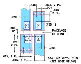
NOTES: 1. TRACE WIDTH IS SHOWN FOR ROGERS RO4350B WITH DIELECTRIC THICKNESS .030" ± .002"; COPPER: 1/2 02. EACH SIDE. FOR OTHER MATERIALS TRACE WIDTH MAY MEED TO BE MODIFIED. 2. BOTTOM SIDE OF THE POB IS CONTINUOUS GROUND PLANE.
